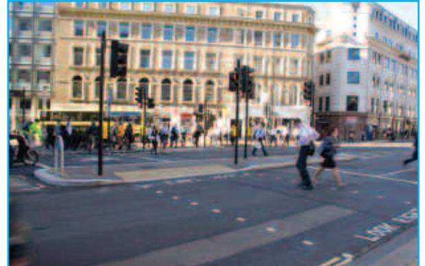
Staggered signalised crossing without guardrail
