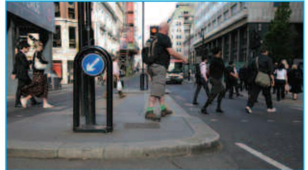
Sign to diagram 610 mounted on hoop top frame.
