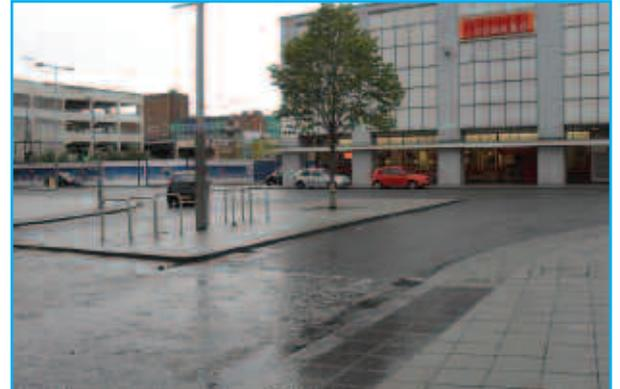
Junction of Corporation Street and Croft Road, Coventry - Junction simplified, traffic signs, bus lane, keep left bollards and guardrail removed, cycle parking on median.
